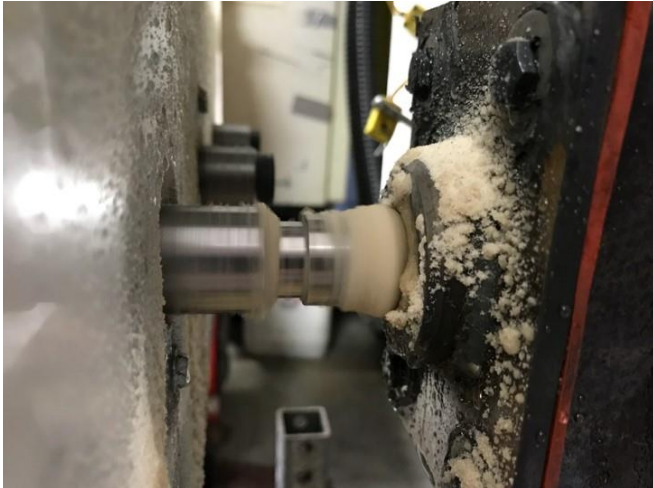
Fig. 2b: Darker shaded sand shows that seal is leaking with uncoated shaft
