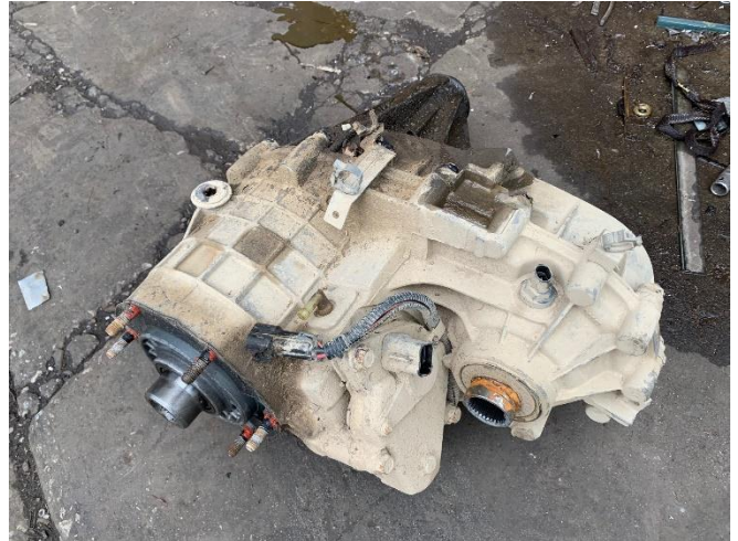
Fig. 1: Power transmission unit scrapped after seal failure
