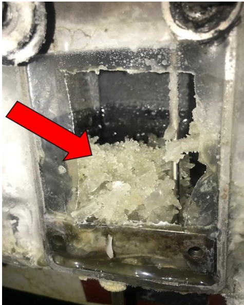
Fig. 11a: Box filled with long ice crystals after uncoated shaft test (R12)
