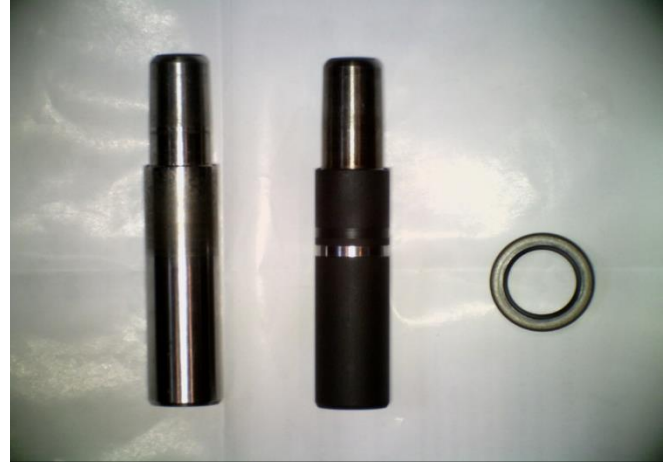
Fig. 8: Uncoated and coated spindles next to .875” SZ seal
