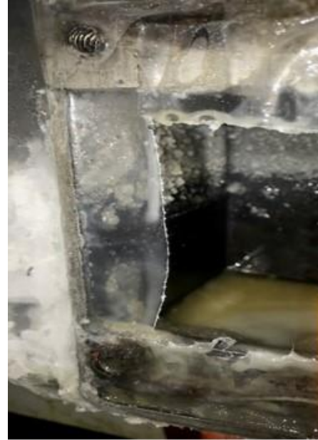
Fig. 11b: Box chamber had minimal ice slush after coated shaft test (R12)
