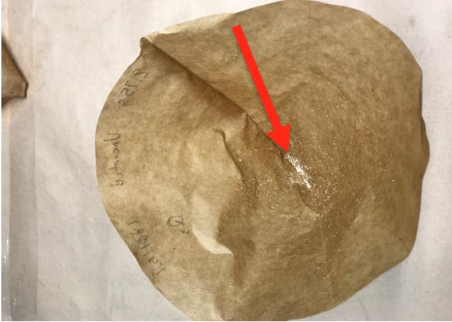
Fig. 10a: Uncoated shaft – sand gets in
